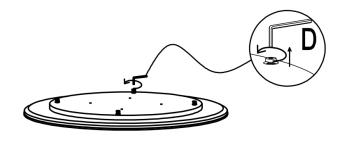
Warning: For safe assembly, please loosen the screws, separate parts 1 and 2, and set all hardware aside before beginning the assembly process
