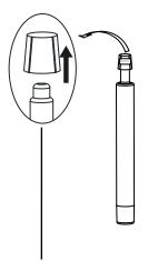
Warning: Before assembly, remove the protective cap from the gas lift column. This cap is only for shipping protection and must be removed for proper function.
